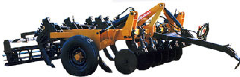
Chisel plough to hitch by pull bar of tractors
