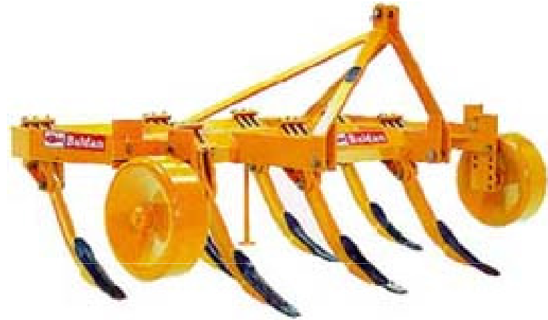
Chisel plough to hitch by 3 points of tractors
